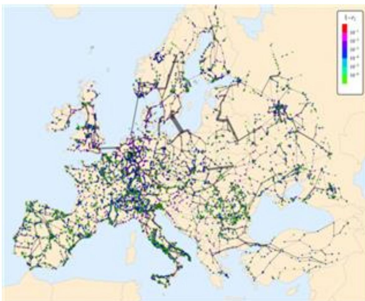
**Figure 7.8.** Local Kuramoto results encoded by the color map as  $1-r_i$ . Red corresponds to low local synchronization, green to high synchronization. The width of gray edges is proportional to the amplitude of the power flow.
